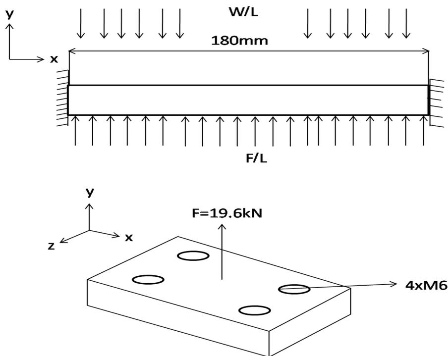
**Figure 6:** Loading State of the Heater Plate and Free Body Diagram of it.
