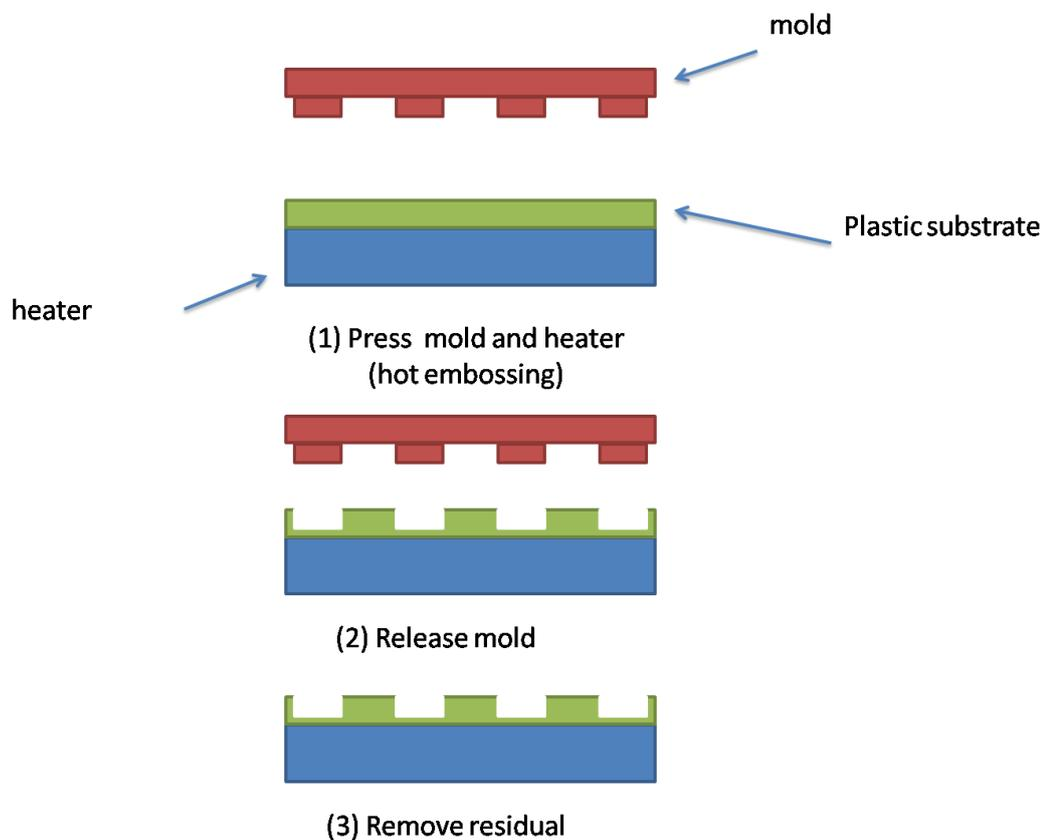
**Figure 4:** Illustration of Hot Embossing for Microfluidic Fabrication
