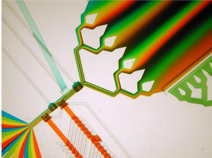
**Figure 1:** Part of a Microfluidic Chip Illustrating Laminar Flow and a Microfluidic Demultiplexer. Channels widths are in the order of 100  $\mu\text{m}$  (Source: Folch Lab, University of Washington).
