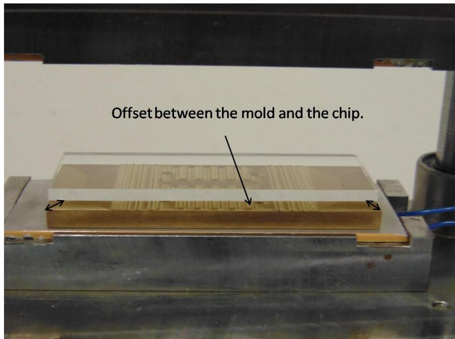
**Figure 14:** The Offset Between the Chip and Mold Edge
