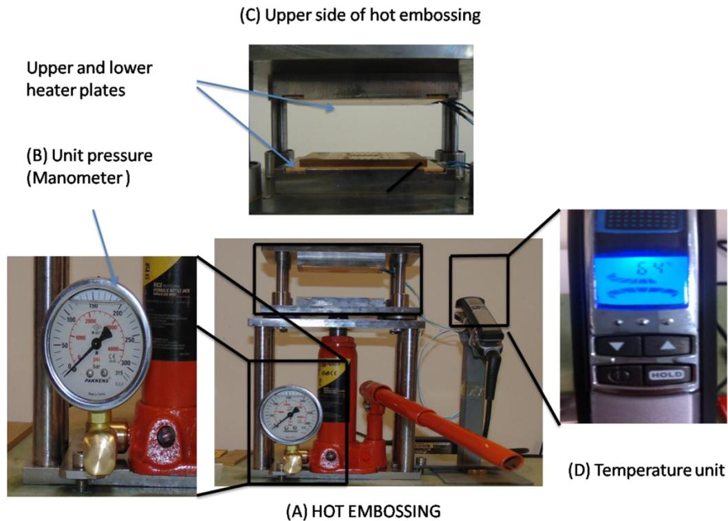
**Figure 5:** Constructed Hot Embossing Press. (a) Overall view of the press (b) Manometer for monitoring the embossing pressure (c) Heater plates (d) Temperature controller unit.
