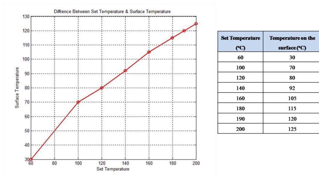
**Figure 11:** Surface Temperature Versus the Set Temperature
