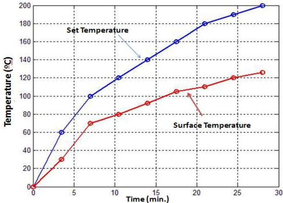
**Figure 12:** Transient Response of the Surface Temperature and the Heater Temperature. The surface temperature of the heater plate was measured with a UNI-T33C multi timer. UNI-T33C has a K type PT100 thermocouple for measuring temperature, and has a precision of 0.1°C .
