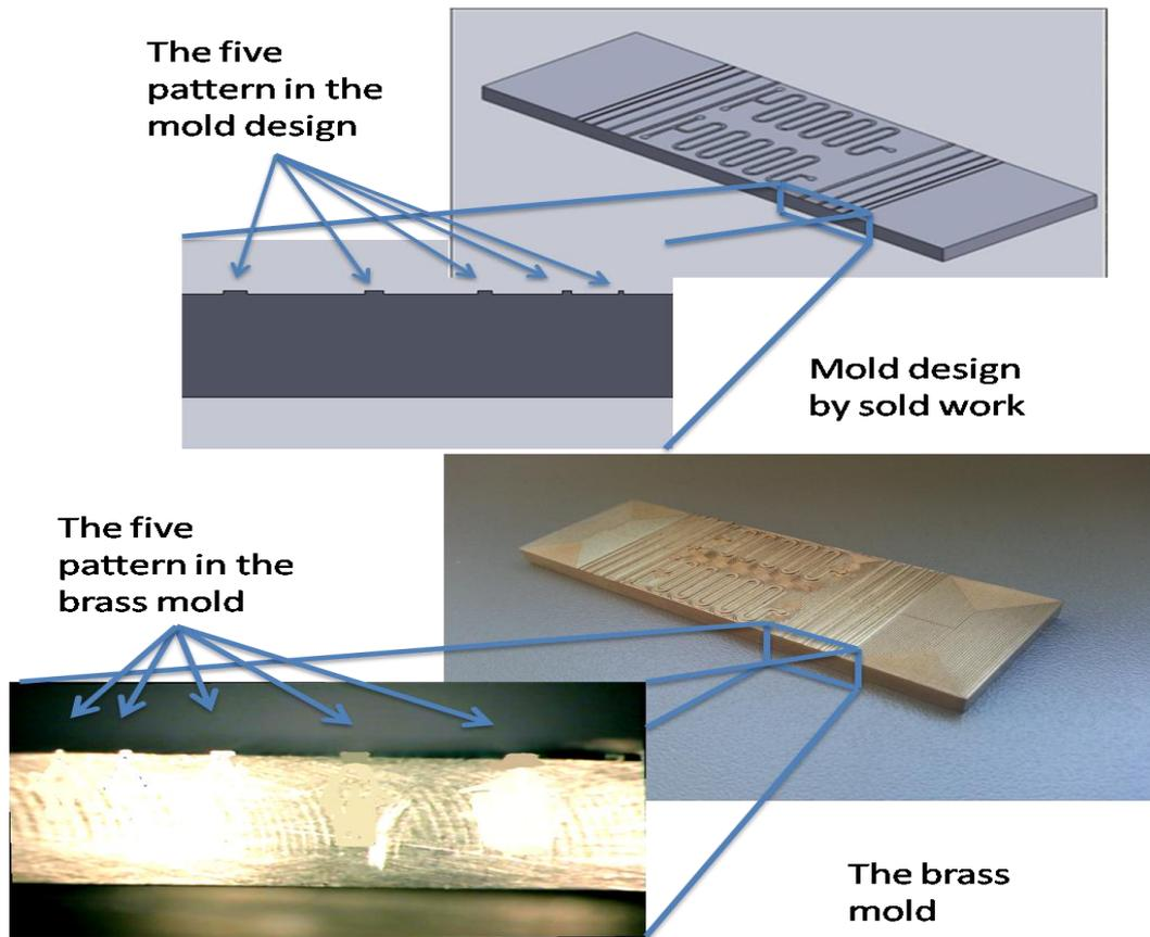
**Figure 9:** The Mold Before and After the Fabrication Process.
