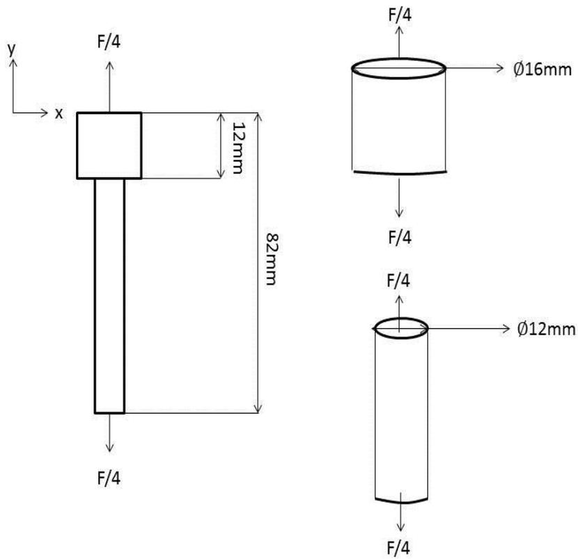
**Figure 7:** Free Body Diagram and the Dimensions of the Upper Cylinder
