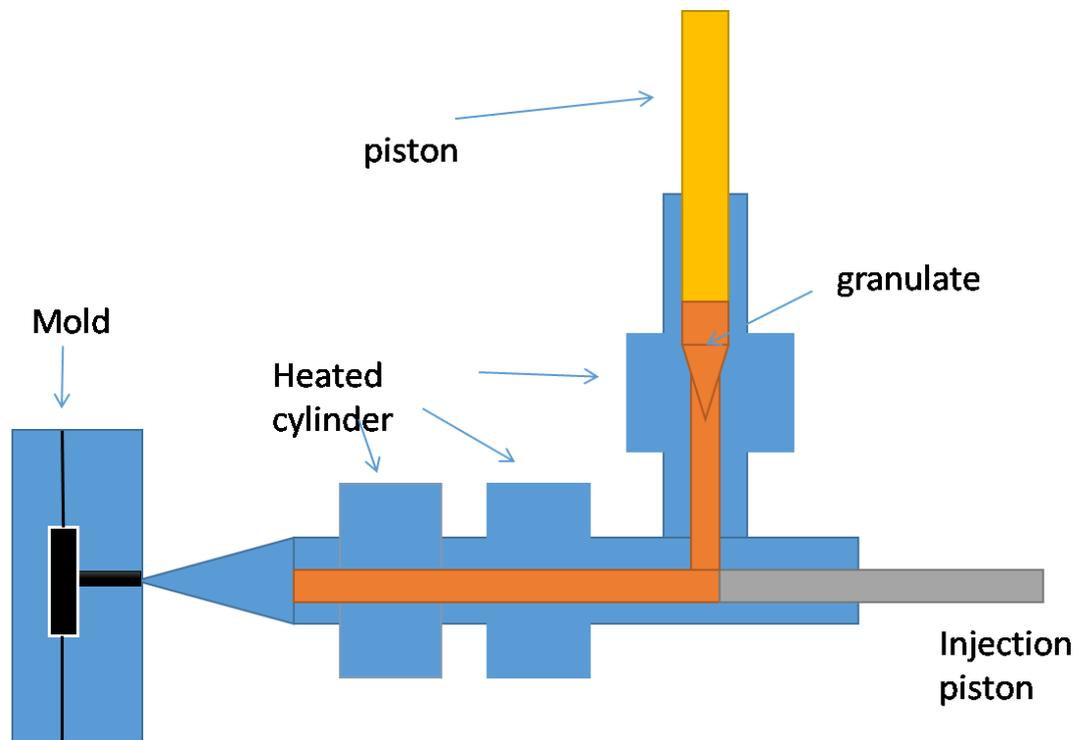
**Figure 3:** Illustration of Micro-Injection Molding.
