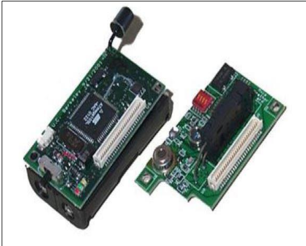
Figure 4 Mica sensor nodes and mica weather board [10]
