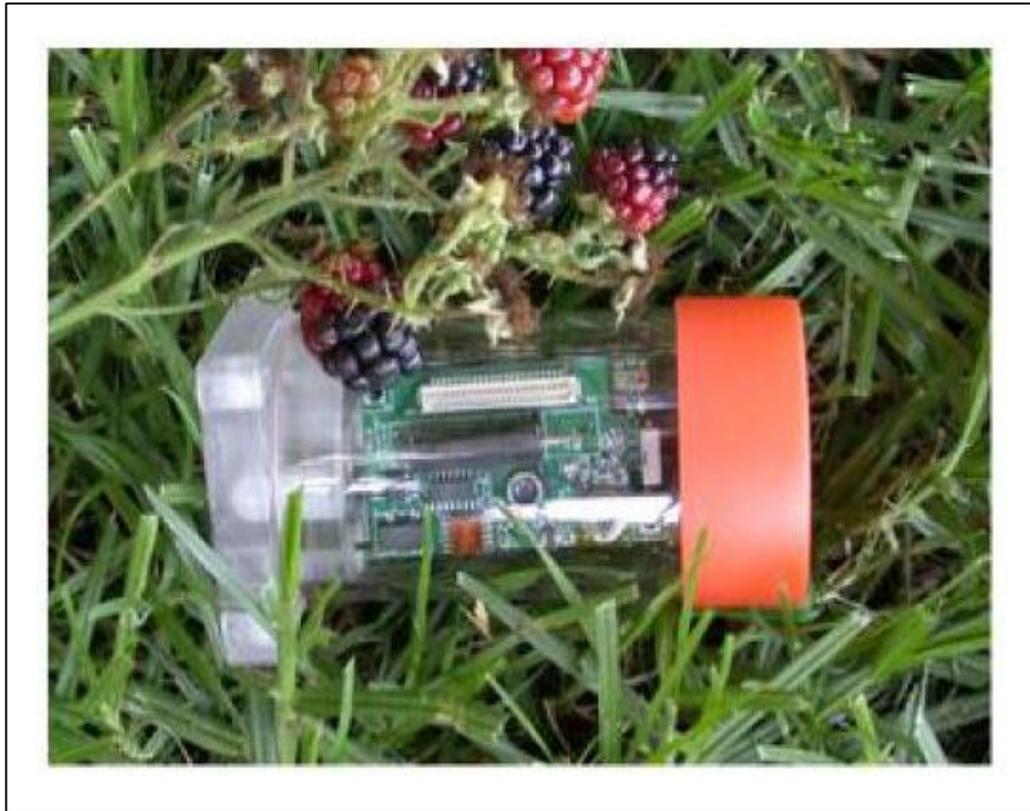
**Figure 3** Deployed sensor node with acrylic fence [17]
