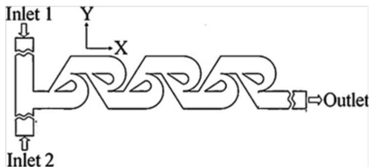
Figure 4: Schematic drawing of one of Tesla type micromixer [19].
