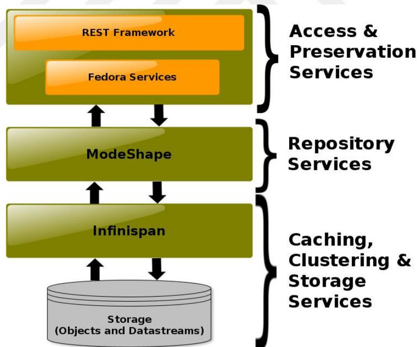
Figure 8 Fedora component stack [63]
