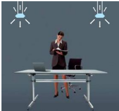
Figure 3.2b. Direct/indirect Lighting (pendant luminaires)
