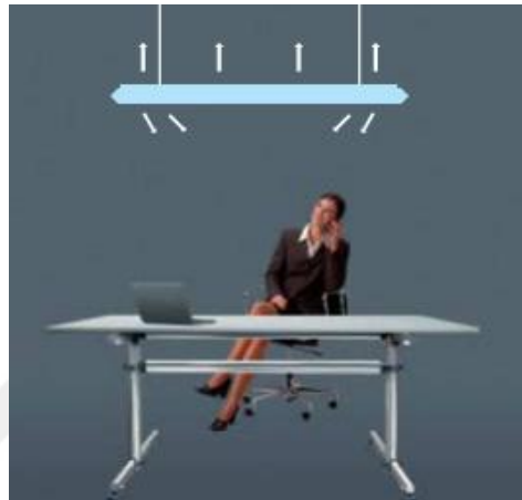
Figure 3.3a. Task Lighting with Special Optical Control
