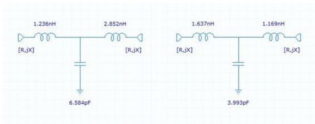
Figure 30 Input and output matching circuits of conventional SSDA
