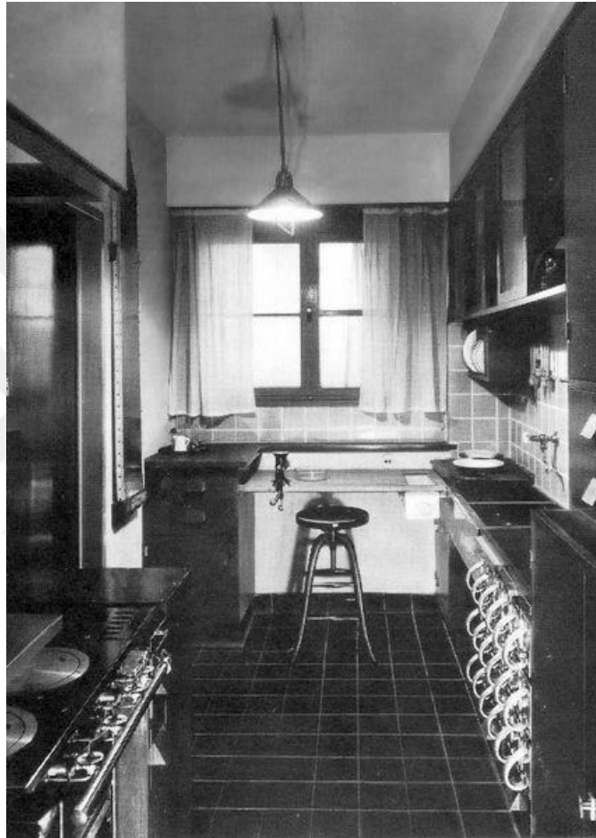
Figure 2. 3: Frankfurt Kitchen Perspective; abundance of natural and artificial light; no decoration, utilized space and efficiency image by Wikimedia Commons ( Filler, n.d. )
