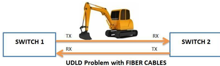
Figure 13 UDLD Problem with Fiber Cables
