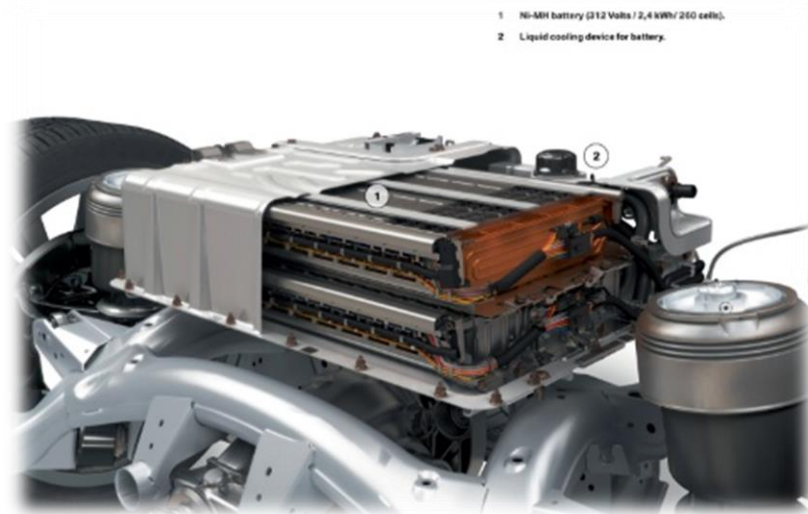
Figure 14 BMW ActiveHybrid X6 high voltage battery pack [44].
