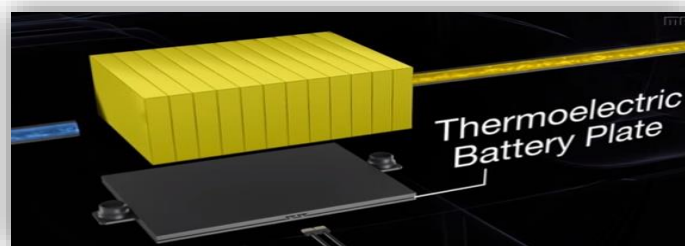
Figure 12 Mahle’s cooling solution using with thermoelectric chips entegreted to the battey pack [38].
