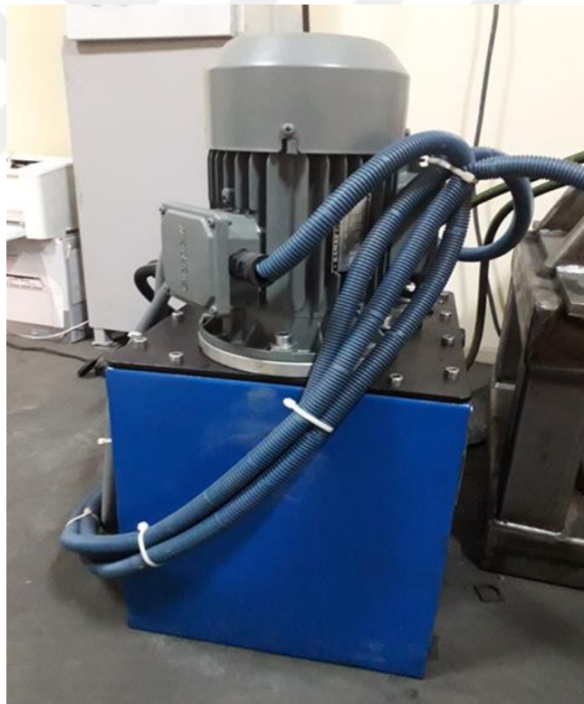
Figure 22: The Hydraulic Power Unit
