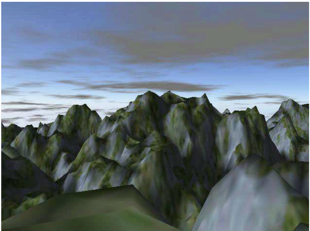
Figure 3.21. Terrain generated with Perlin Noise: harmonics=6 , frequency=1 , amplitude=50
