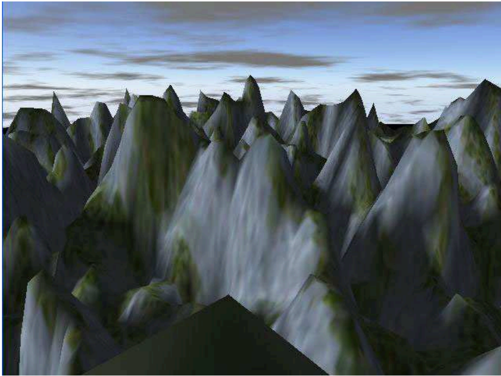
Figure 3.17. Terrain generated with Perlin Noise: harmonics=2 , frequency=0.15 , amplitude=50
