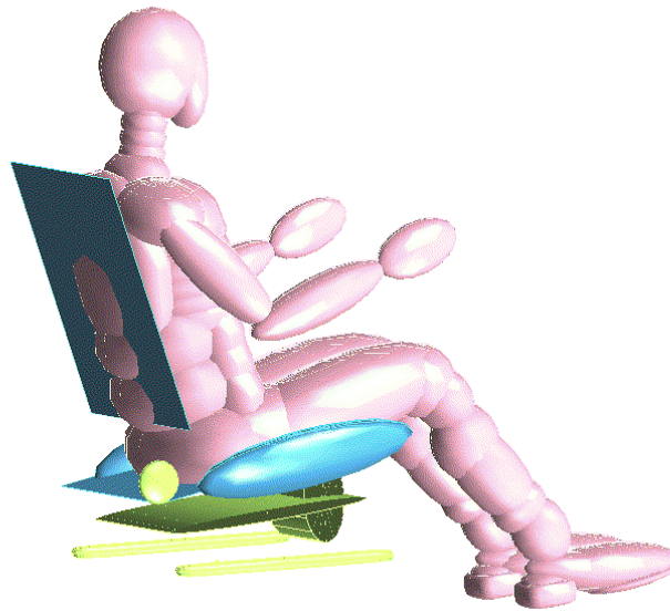
Figure 3.7. Dummy and seat model together (Madymo)
