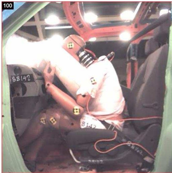
Figure 4.10. Sled test at t = 100 ms
