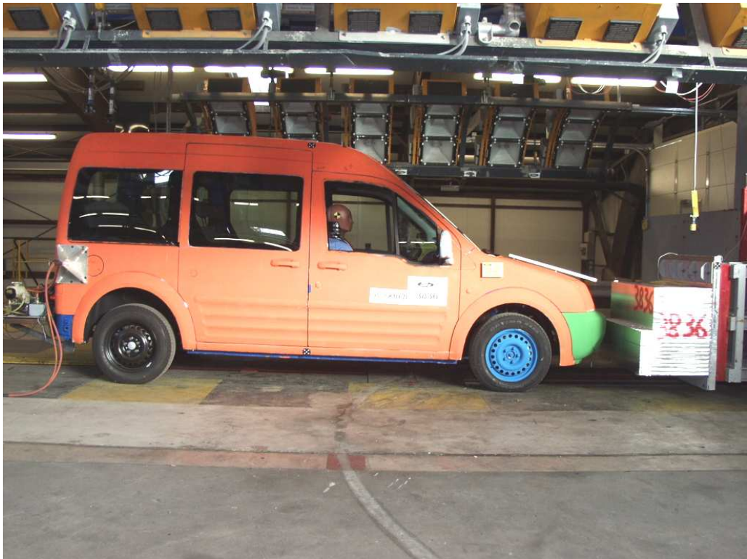
Figure 5.1. Front offset impact test setup for a light commercial vehicle hitting a deformable barrier at a speed of 56 km/h
