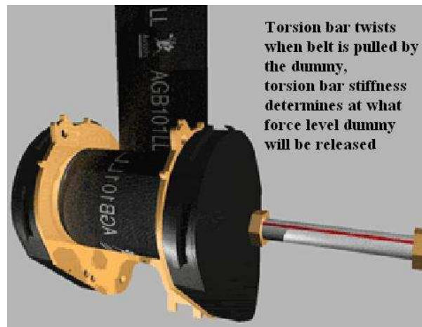
Figure 3.17. Retractor load limiter
