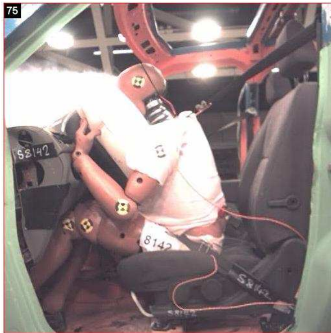
Figure 4.8. Sled test at t = 75 ms
