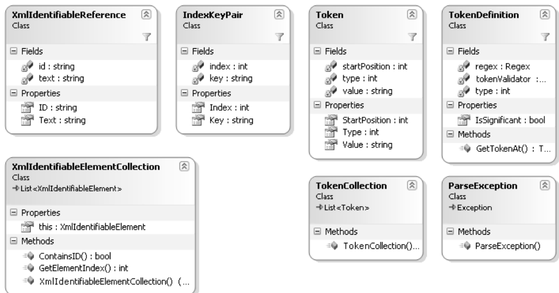
Figure A.5. Code Checker class diagrams - V
