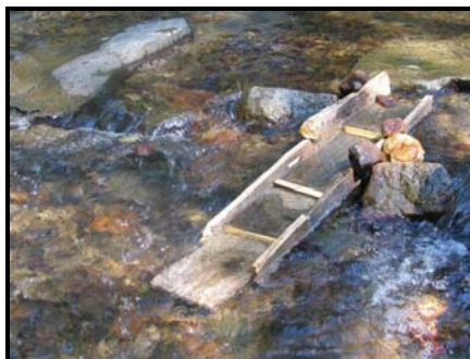
Figure 5.9. Sluice used for magnetite enrichment
