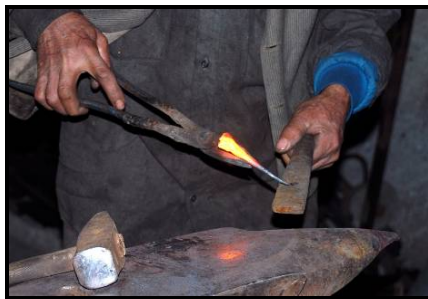
Figure 5.49. Fitting the iron piece into the "nail iron"
