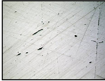
Figure 5.55. Microstructure of nails at Ömerli from bloom iron (06/105)
