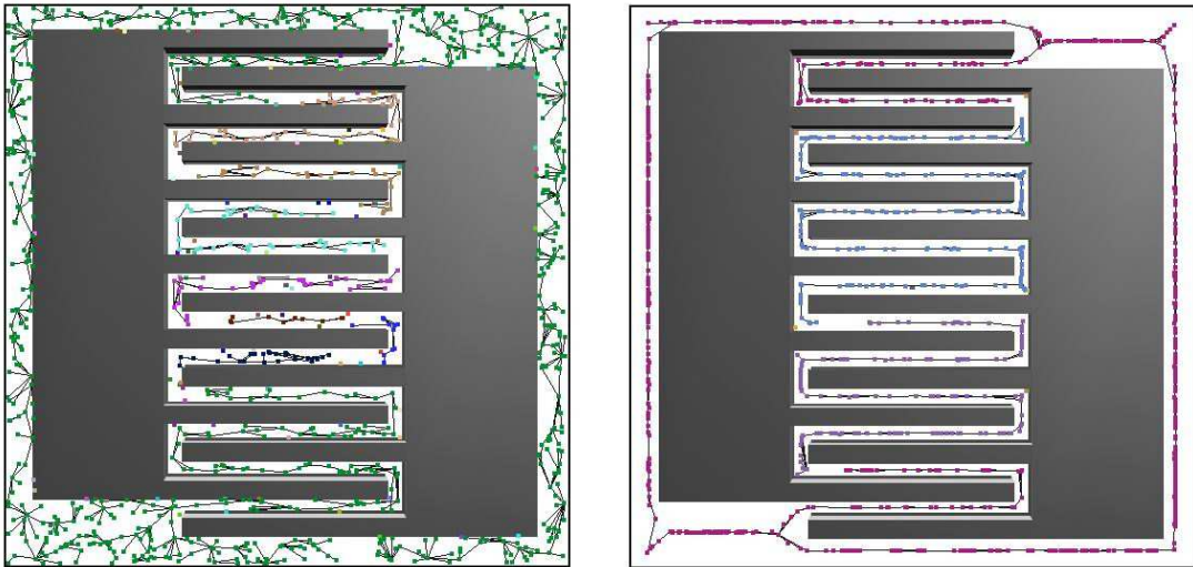
Figure 3.5. Two sampling strategies in maze a. Uniform sampling method, b. Sampling on Medial Axis of the Free Space method [28]
