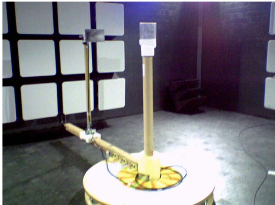
Figure 4.4. Aluminum flat plate located at turntable in anechoic chamber
