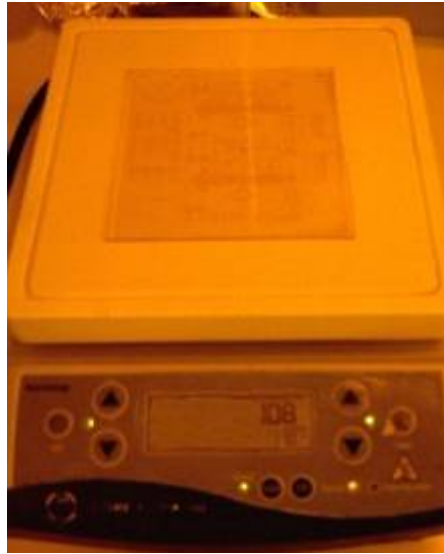
Figure 2.12. After developing the photoresist, the wafer is hard baked at 110°C on hot plate
