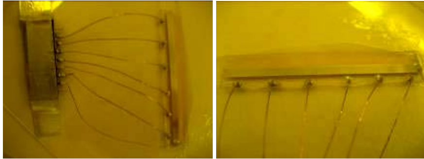
Figure 2.30. Wired and encapsulated PLED samples
