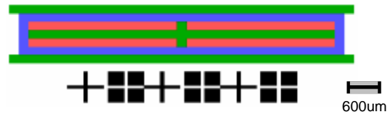
Figure 2.8. Alignment marks for four layer micro fabrication process
