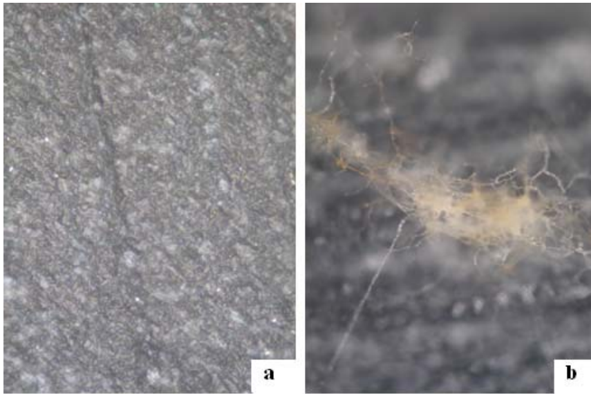
Figure 4.27 Optical Microscope images of the Nanocomposites Before (a) and After (b) the LB Medium study
