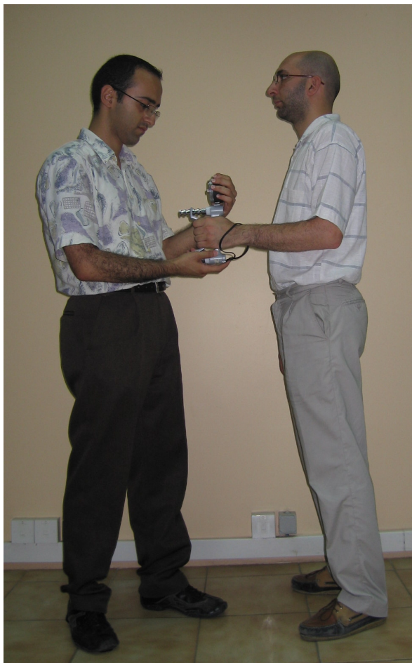
Figure 4.11. Measurement of grip strength value of left hand while the subject is standing and dynamometer is supported
