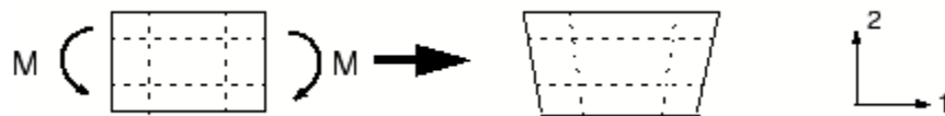
Figure 4.7. Deformation of a fully integrated, linear element subjected to bending moment M
