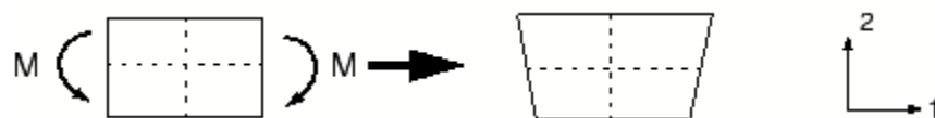
Figure 4.8. Deformation of a linear element with reduced integration subjected to bending moment M
