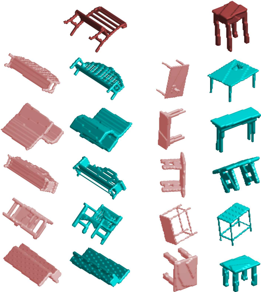
Figure 6.13. Class-based ARR selection for bench seat and rectangular table classes. The top red figures are the reference models. Pink figures at the left are the outputs of CPCA-based normalization. Cyan figures under the reference models are the best choice out of the 48-ARR representations.
