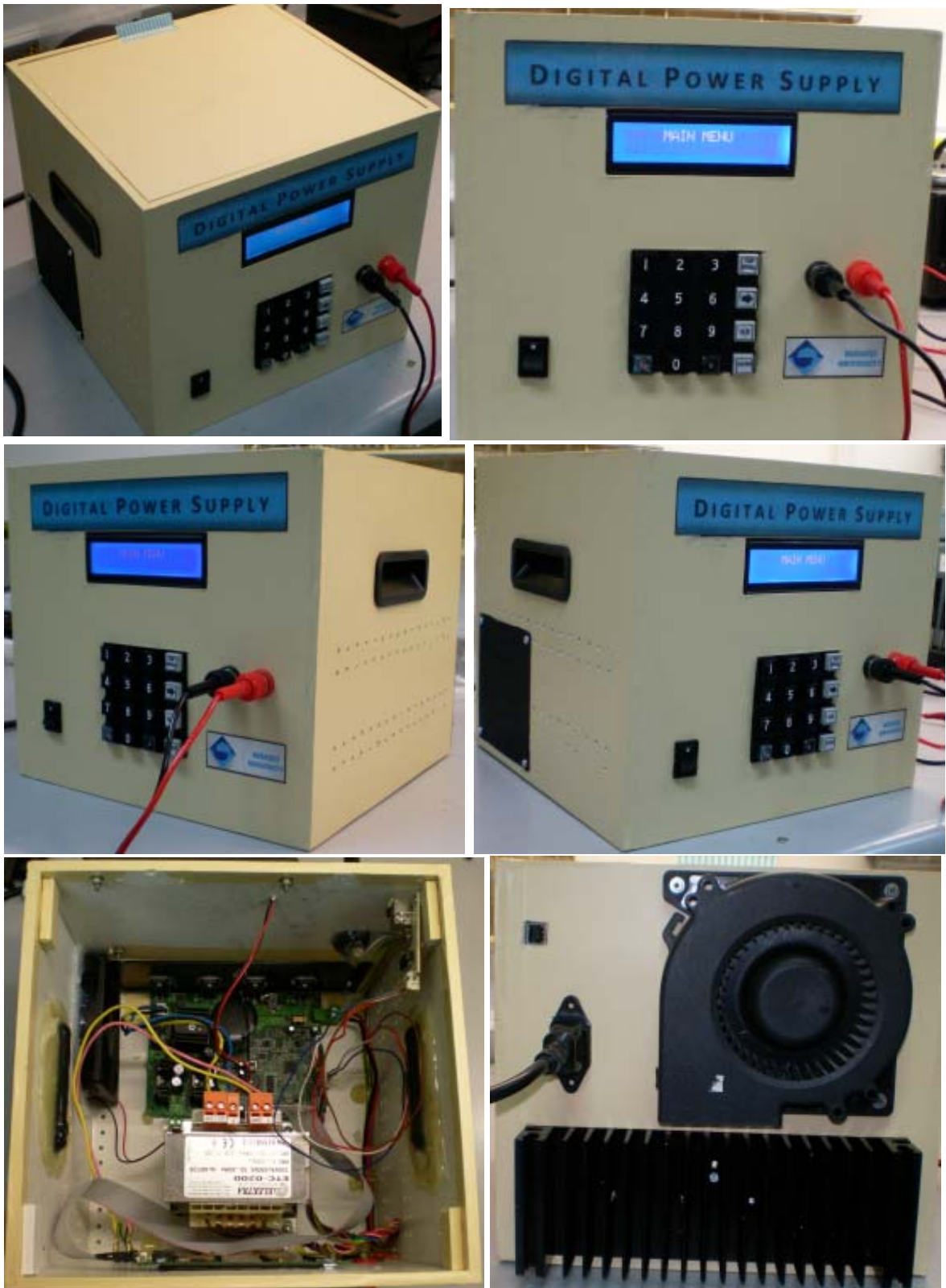
Figure 4.2. The power supply from various angles
