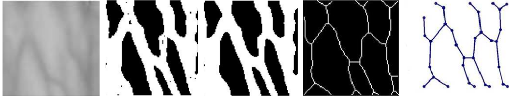
Figure 3.11. LEM extraction steps: Vein image, Yasuda binarization, noise removal, skeletonization and line segments generation
