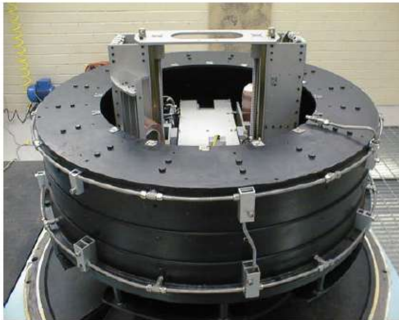
Figure 5.3. Drum Centrifuge Test Machine.
