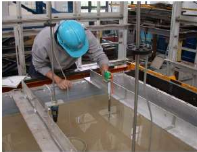
Figure 4.6. Measurement of the settlements after liquefaction test (Ueng et al. 2009).
