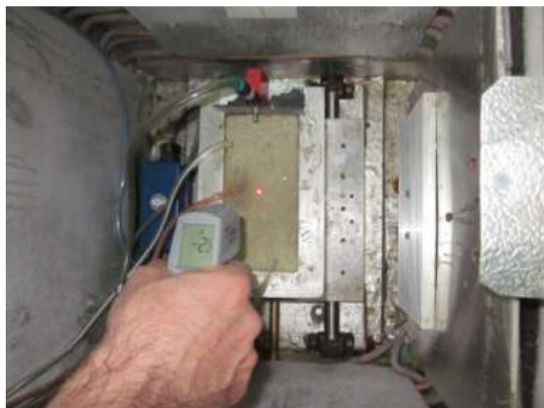
Figure 7.71. Sand specimen tested under 0°C.
