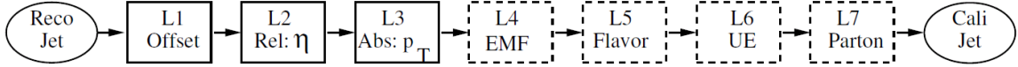
Figure 5.17. Schematic picture of a factorized multi-level jet correction, in which corrections to the reconstructed jet are applied in sequence to obtain the final calibrated jet. Required correction levels are shown in solid boxes and optional correction levels are shown in dashed boxes.
