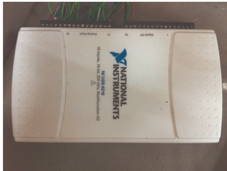
Figure 4.5. The data acquisition system of LabVIEW.
