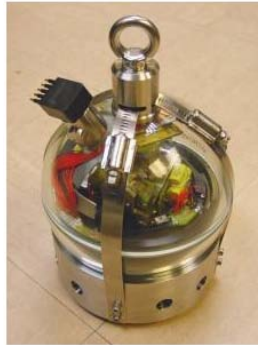
Figure 1.7. The CMG-40 TOBS Ocean Bottom Seism. build by Güralp Sytem Ltd [4] .
