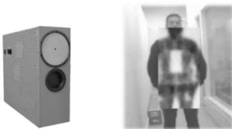
Figure 1.11. Illustration of concealed object by ThruVision TS4 [22].
