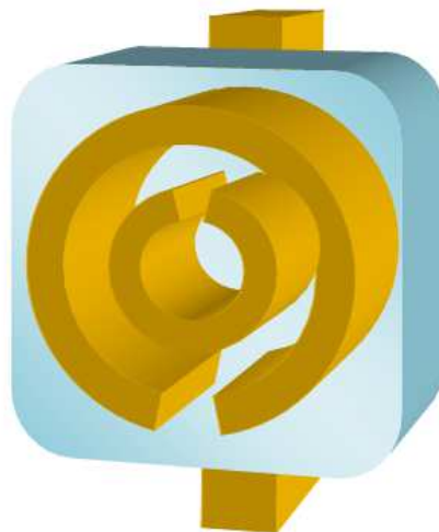
Figure 1.7. Combinations of SRRs and wire as LHM.
