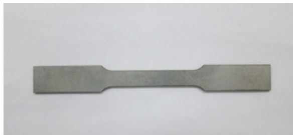
Figure 5.2. The specification of dog-bone test specimen cut in transverse direction.
