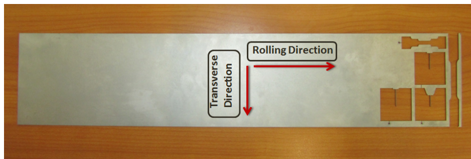
Figure 5.1. Parent sheet of NiTi and illustration of rolling and transverse directions on it.
