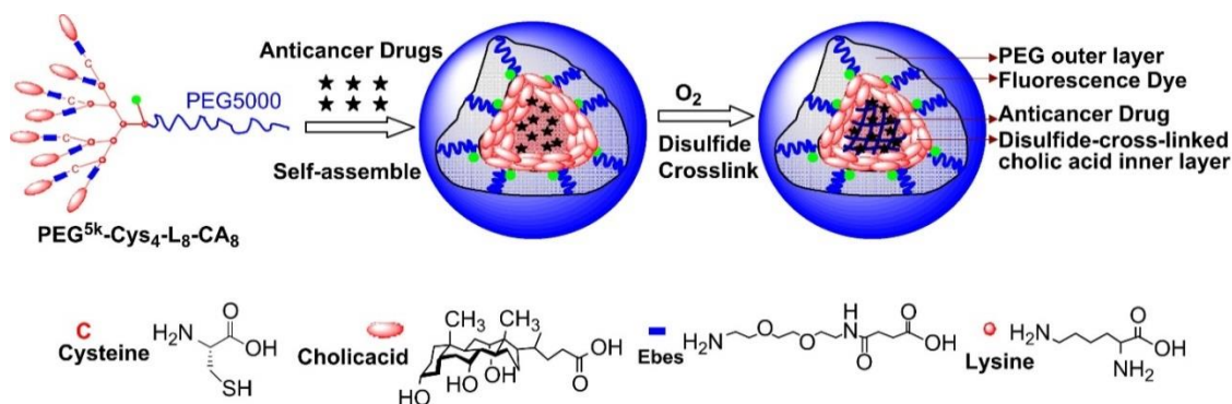
Figure 1.12. The disulfide crosslinked micelles formed by oxidation of thiolated dendron polymer after self-assembly [50].
