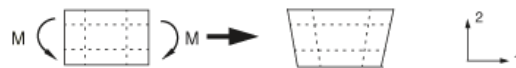
Figure 4.8. Deformation of a fully integrated, linear element subjected to bending moment M [56].
