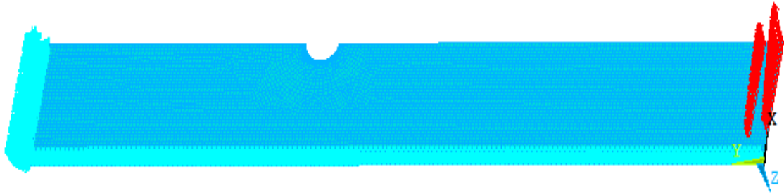
Figure 5.10. The torsional load and displacement boundary conditions.
