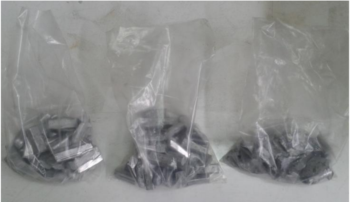
Figure 3.16. Master ingots cut into pieces to be used later in the phase 1-b and phase 2-b.
