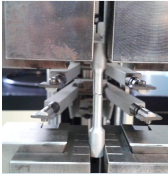
Figure 3.25. The specimen fractured under tensile test.
