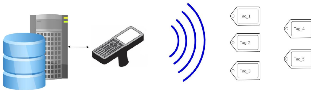
Figure 1.1. A typical RFID system
