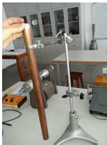
Figure 2.8. Measurement of the Time of Magnet Fall Inside the Copper Tube.
