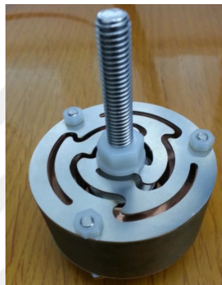
Figure 3.16. Measured Resonator with Small Ring Magnet Inside.
