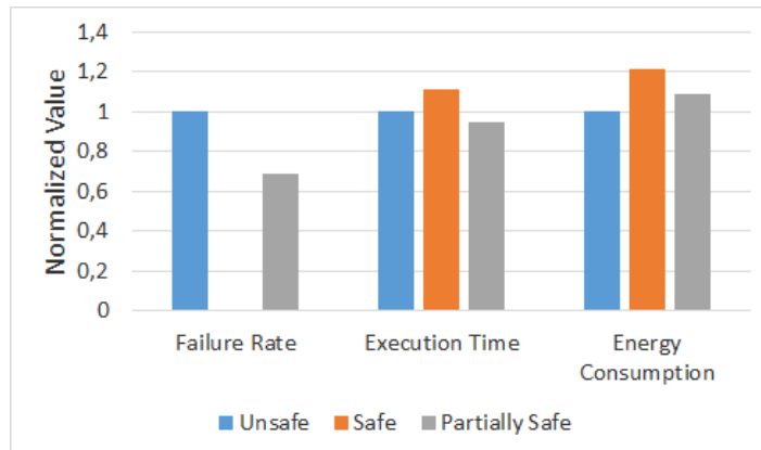
Figure 4.12. Normalized values of failure rate, execution time and energy consumption for the Susan corners application.
