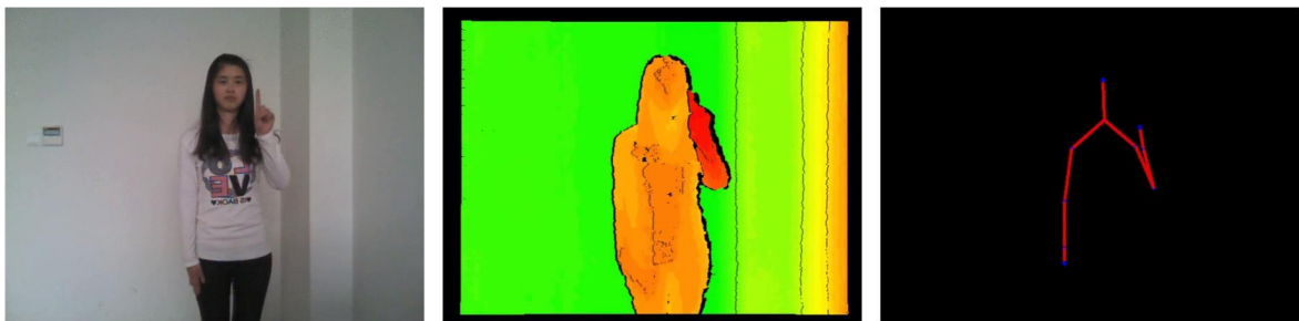
Figure 2.4. An example sign video from DEVISIGN dataset [5]. Left to right; RGB video, visualized depth map and body pose information
