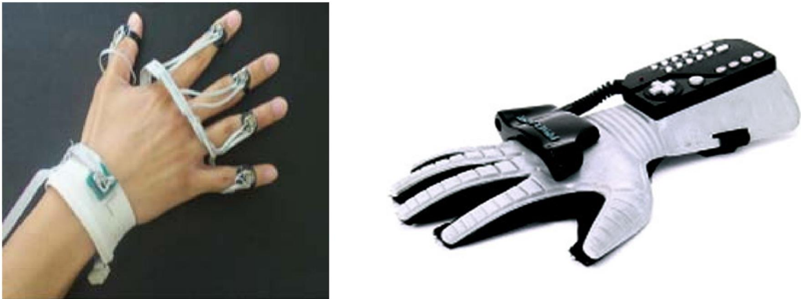
Figure 2.1. Sensors used in earlier research on sign language recognition. Left: PowerGlove [1], Right: Accele Glove [2]
