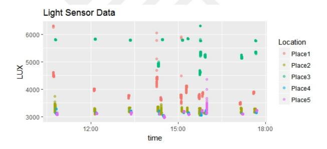
Figure 4.24: Lux sensor data from office
