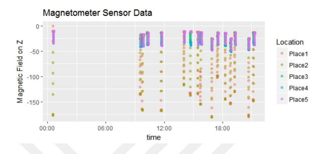
Figure 4.18: Magnetic field data on Z-axis from living room
