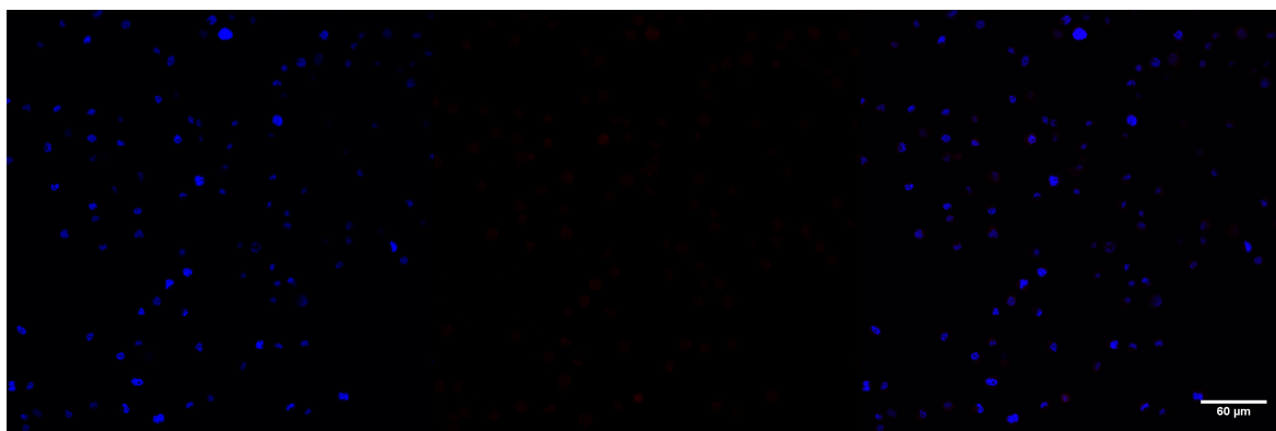
Figure 5.7. Photoconversion of DAPI and MMP680 probe in the Thp-1 cells. Note that the excitation/ emission were 638 nm/643-717 nm
