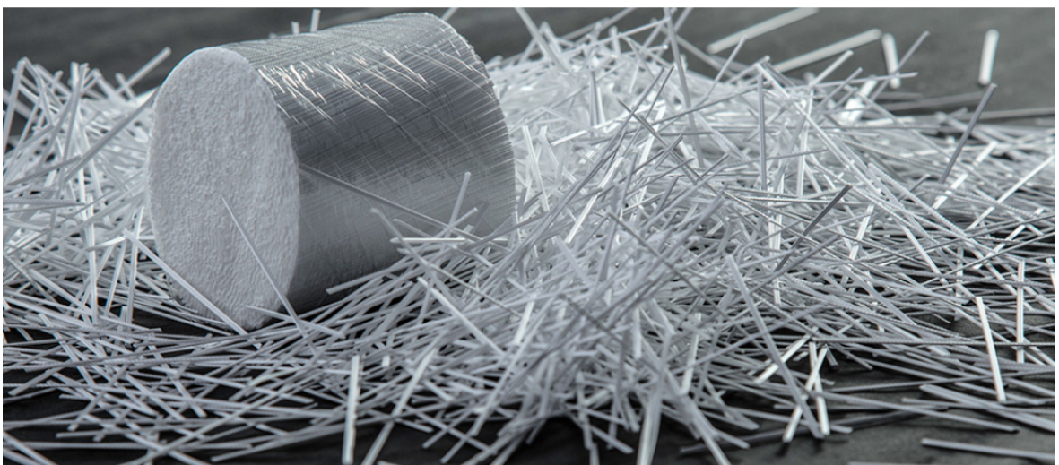
Figure 3.2. Structural macro - synthetic fibers
