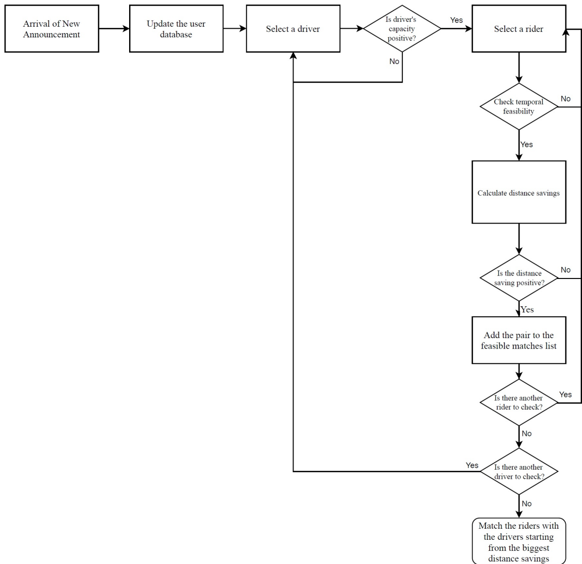
Figure 5.2. Flowchart of the weighted bipartite ride-matching algorithm.
