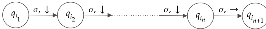
Figure 4.2. A part of the transition diagram of a one-way deterministic blind counter automaton
