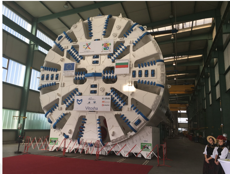
Figure 5.11. EPB TBM Cutterhead used in the Project.
