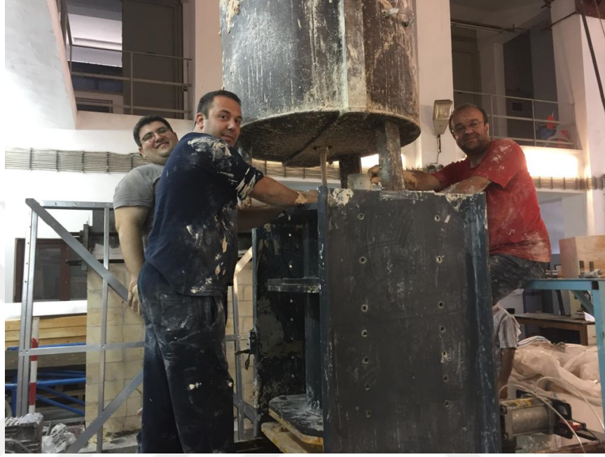
Figure 3.2. Clay Slurry Placement.
