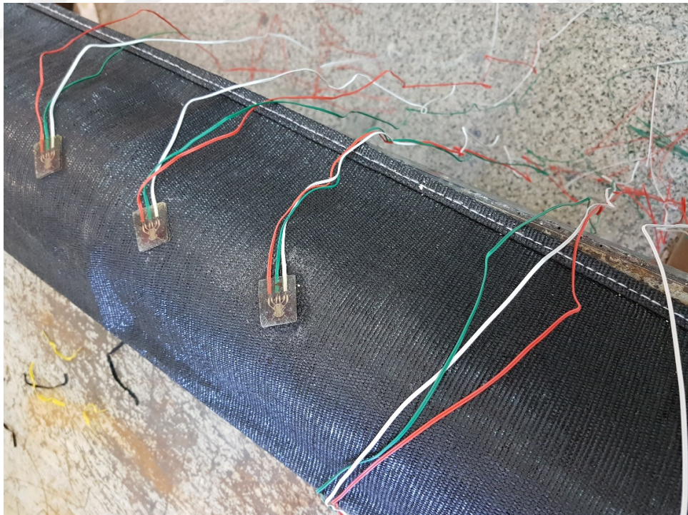
Figure 3.11. Strain Rosettes glued onto a geotextile encasement.
