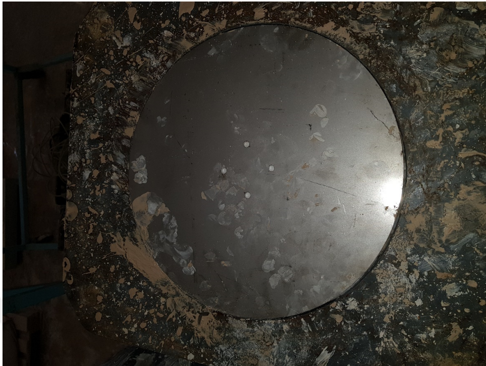
Figure 3.10. The Stainless-steel on the top of Geotextile Filter.
