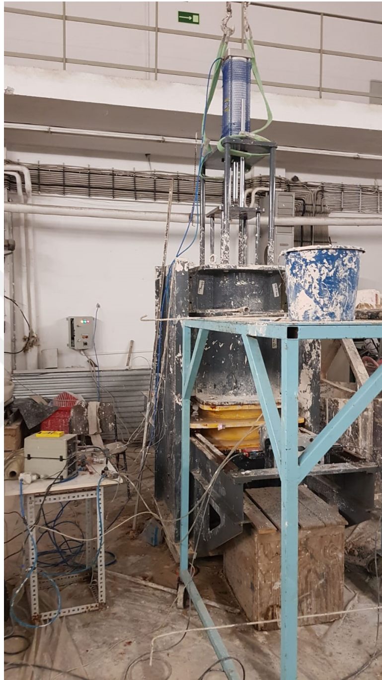
Figure 3.14. Taken Before Cyclic Shearing Begins.
