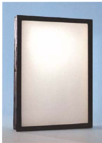
Figure 2.38: Glass sample with black edging and aerogel-filled glazing cavity. (Leydecker, 2008).
