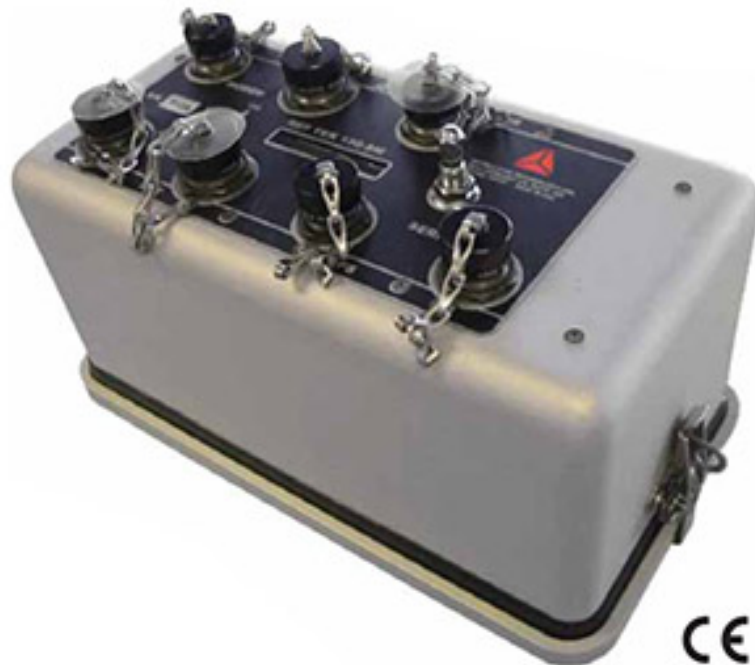
Figure 2.3. View of the 24-bit strong motion accelerograph [5]
