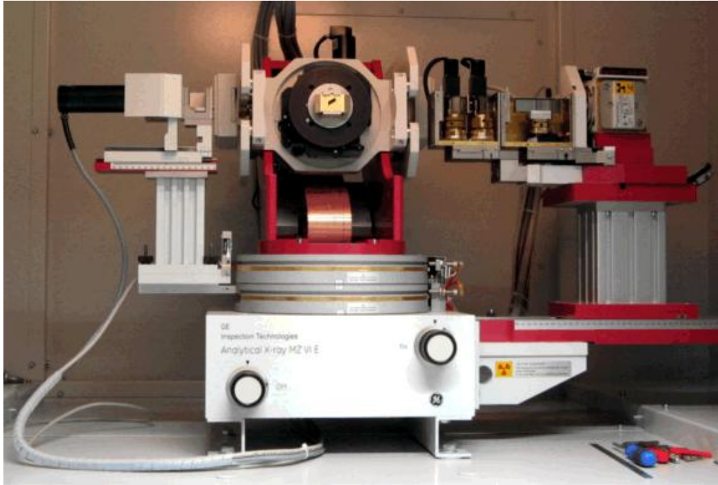
Figure 3.8. Residual stress measurement with XRD.
