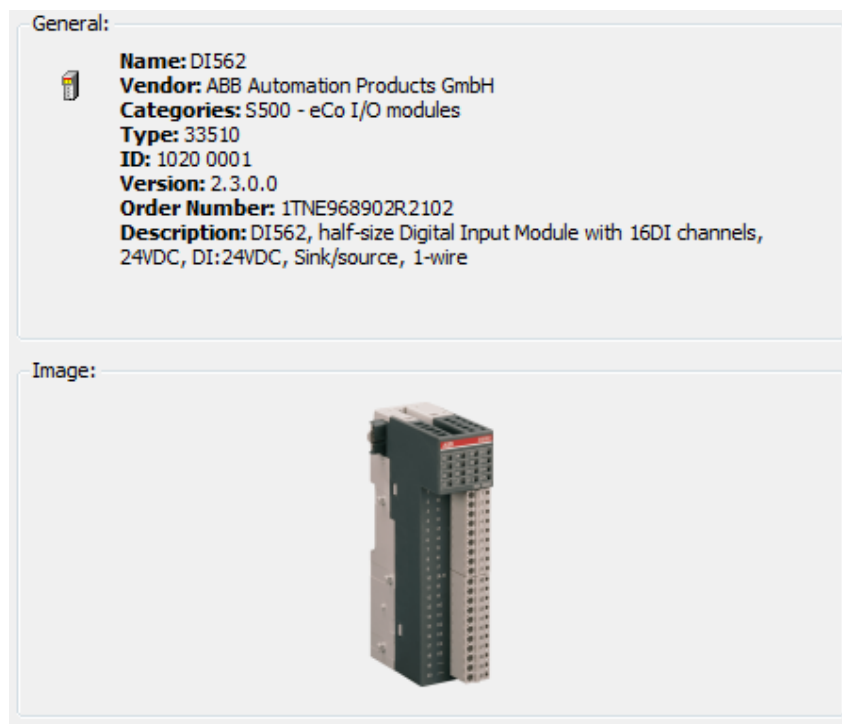
Figure 4.8 Specifications of DI562 module
