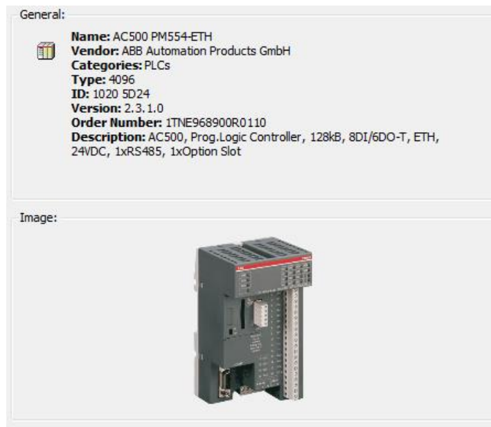
Figure 4.7 Specifications of AC500 PM554-ETH
