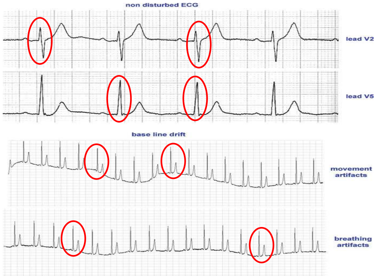
Figure 2.6 Low frequency noises present in ECG signal [29]
